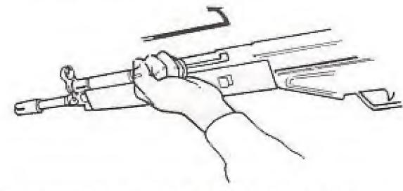
2. Remove the magazine and set the selector lever on "S" or "Safe"; then check the rifle to make sure it is unloaded. To inspect the SAR-3, unfold the cocking handle located on the left side of the rifle at the front of the handguard and pull the cocking handle towards you (rearward); then
